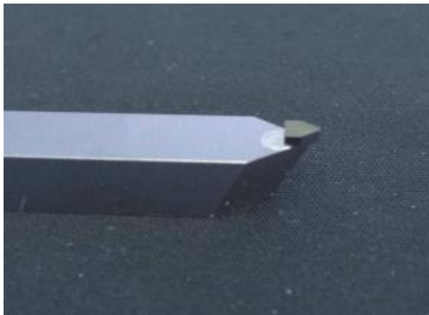
PICTURE 1: Digital pictures of a tooling tip with a diamond insert at its extremity
