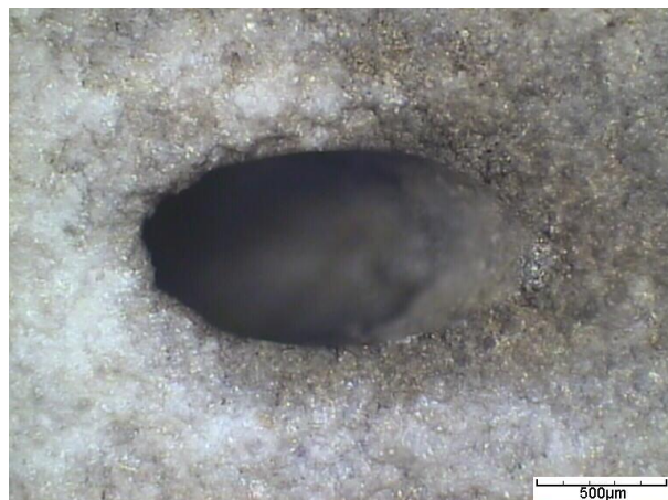
PICTURE 5B: Microscope image of a hole with 0.35mm radius (frontside, thin coating)
