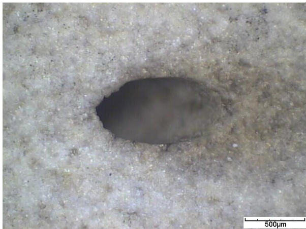
PICTURE 4A: Microscope image of a hole with 0.25mm radius (frontside, thick coating)
