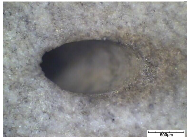
PICTURE 4B: Microscope image of a hole with 0.35mm radius (frontside, thick coating)
