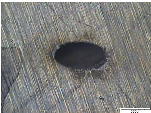
PICTURE 4C: Microscope image of a hole with 0.25mm radius (backside, thick coating)
