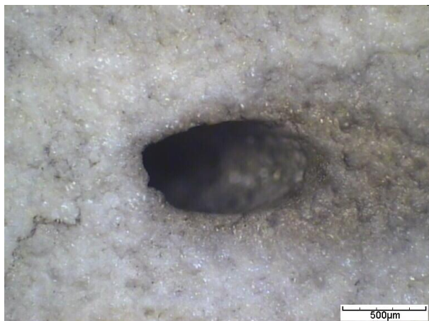
PICTURE 5A: Microscope image of a hole with 0.25mm radius (frontside, thin coating)
