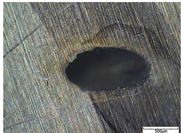
PICTURE 4D: Microscope image of a hole with 0.35mm radius (backside, thick coating)
