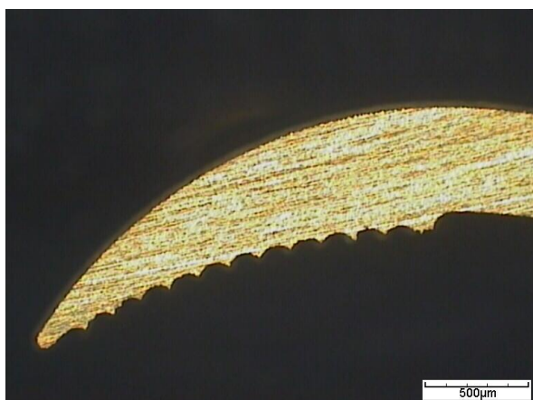
PICTURE 25: Microscope image of the backside (dark field illumination)
