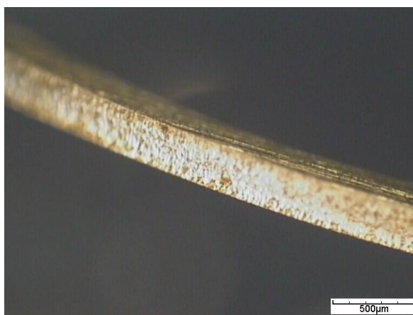
PICTURE 27: Microscope image of sidewall (dark field illumination)
