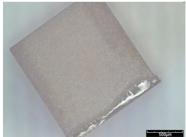
FIGURE 5: Side view of a cubic zirconia cube after the cut in the "cross" direction. Around 15% of the total thickness is not cut through. The cube has been separated from the rest of the bar by breaking this remaining part.
