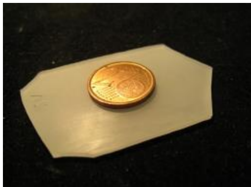
FIGURE 1: Cubic zirconia plate to be cut into small cubes.
