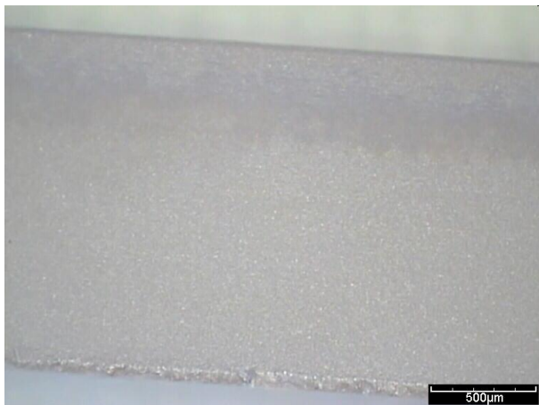
FIGURE 4: Side view of a cubic zirconia bar after the cut in the first direction.
