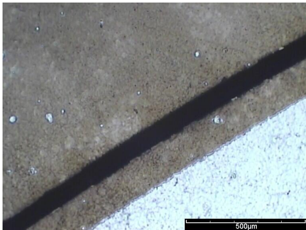
FIGURE 2: Microscope image of the cut (bright field imaging). The edge of the disc is sharp and clean.
