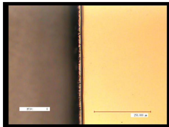
PICTURE: Microscope image of SIC after processing (bright field illumination; top view with high magnification)
