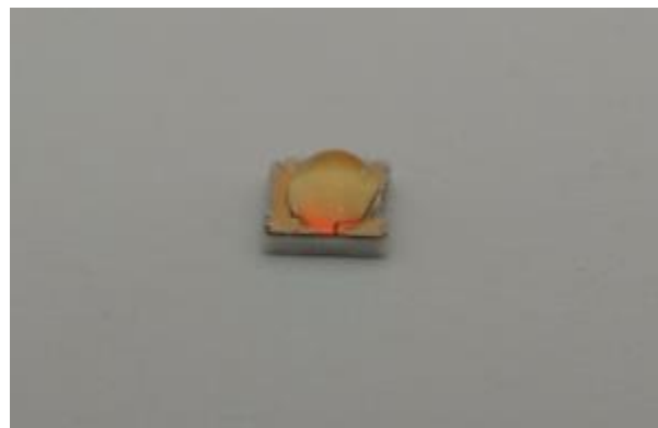
PICTURE 2: Digital picture of one cut chip (3.4 x 3.4 mm) (dark field illumination; frontside view)
