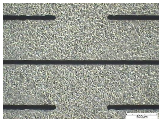
PICTURE 6: Microscope image of the “750micron” sample (dark field illumination, backside view)
