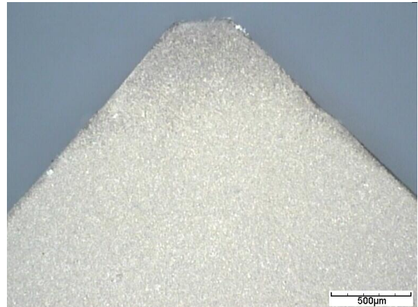
PICTURE: Microscope image of the back side edge (dark field illumination; bottom view)
