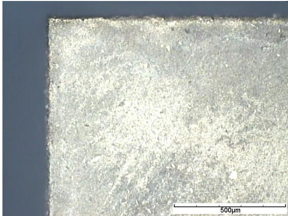
PICTURE: Microscope image of front side edge (dark field illumination; top view)
