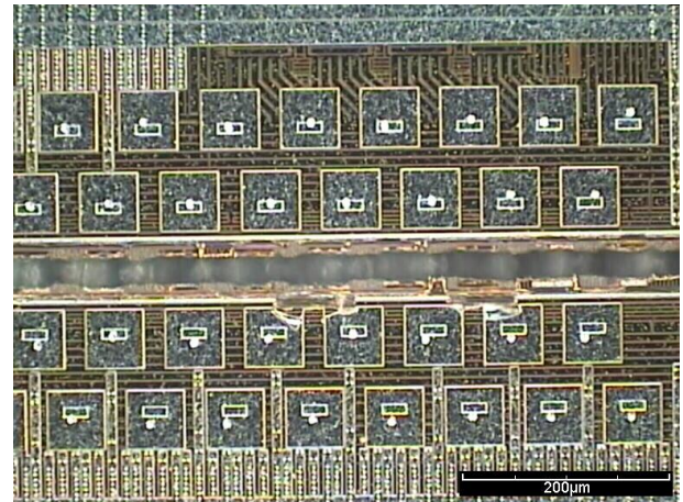
PICTURE 2-6: Microscope image of a line cut into the silicon wafer with the 30µm nozzle. (dark field illumination)
