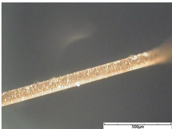
PICTURE 5: Edge view of work piece C, 1.4mm/s.
