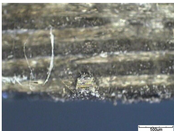
PICTURE 6C: Image of the top of the cut wall of part 18, showing a very small bridge.
