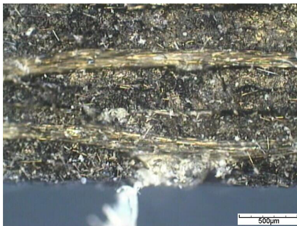
PICTURE 4: Image of the bottom of the cut wall of part 12, below a cut sewing thread, showing a very small bridge.
