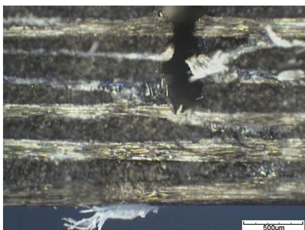
PICTURE 6E: Cross-section of the line grooved with 10 passes.
