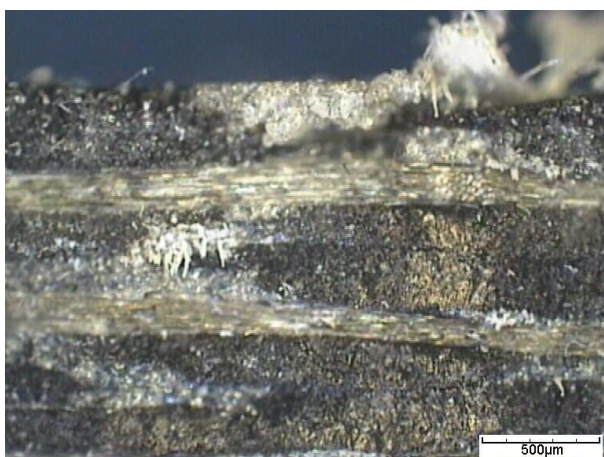
PICTURE 3C: Image of the top of the cut wall of part 11, where the sewing thread was cut.
