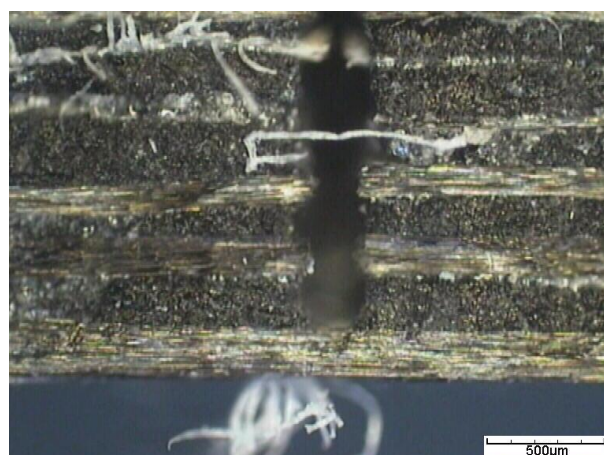
PICTURE 6F: Cross-section of the line grooved with 15 passes, close to the bottom.
