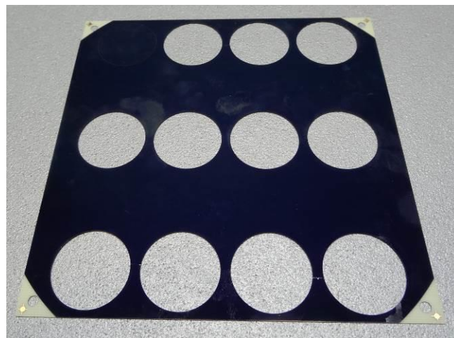
FIGURE 3: Picture showing the front side structure on Anonymous type cells and on C60 Sunpower cells (circular shapes already cut)
