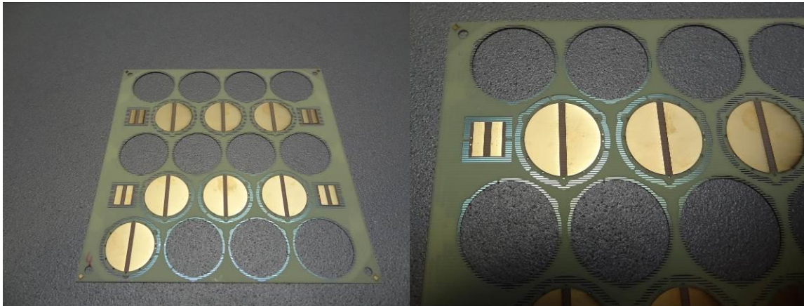
FIGURE 2: Pictures showing the backside structure on Anonymous type cells (circular shapes already cut)
