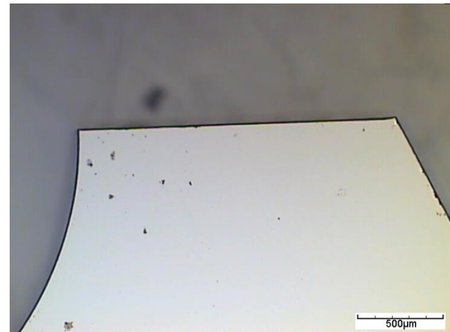
PCD beam entry side: Note - minimal edge chipping
