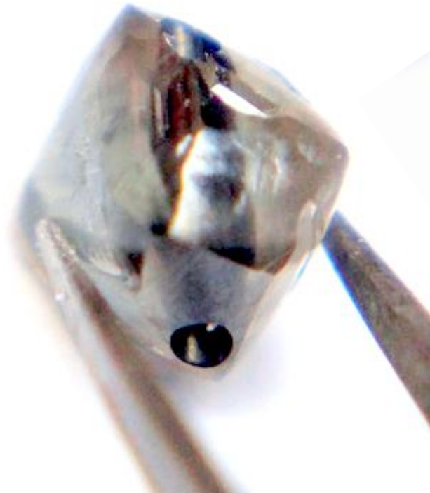
Diamond with 1.0mm hole - parallel sided
