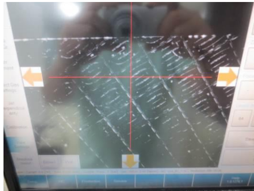
PICTURE 2: The lighting system could be helpful to see the line for the alignment.
