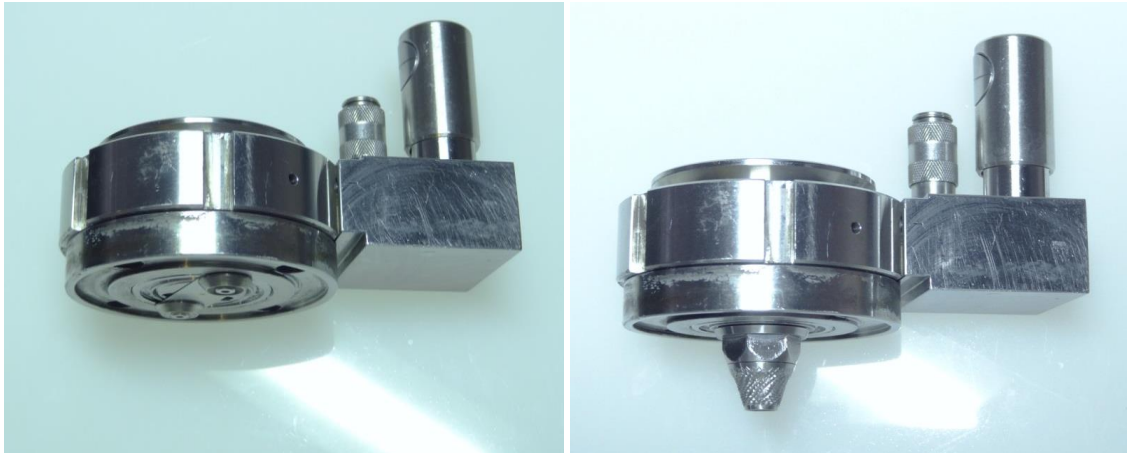
FIGURE B: Coupling unit setups used with the 30µm nozzle (left) and the 50µm nozzle (right)
