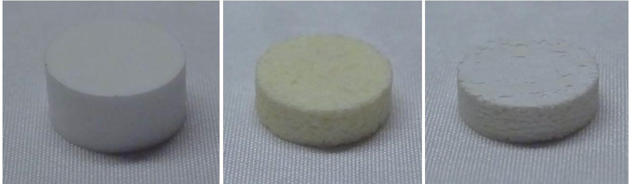
PICTURES 1A, 1B & 1C: Camera pictures of the cut discs; left: fine zirconia, center: rough zirconia; right: CMC.
