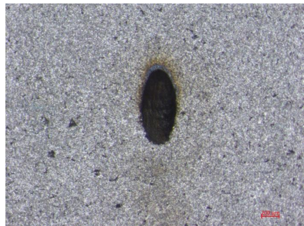
FIGURE 8C: Microscope image of the back side of a diffuser hole (0.4mm diameter)
