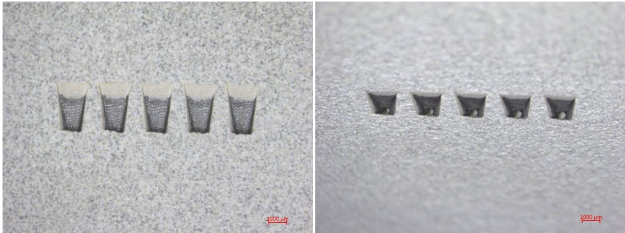
FIGURE 8 A&B: Microscope images of the front side of the diffuser holes drilled in the coated plate
