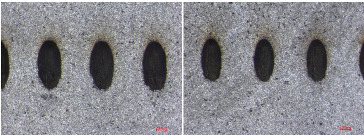
FIGURE 7 C&D: Microscope images of the front side of the holes drilled in the coated plate (left: 0.5mm, right: 0.4mm)
