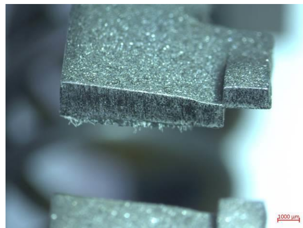
PICTURE 2E&F: Microscope images of the cut walls of another ring cut with a 80µm nozzle
