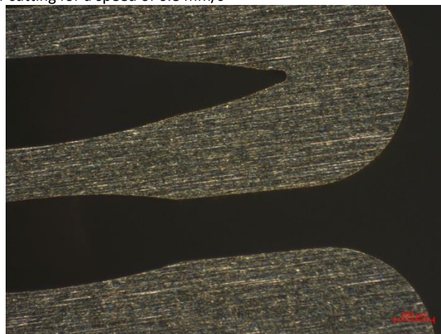
PICTURE 4 and 5: Picture of the pattern for a speed of 1.2 mm/s, frontside at left and backside at right
