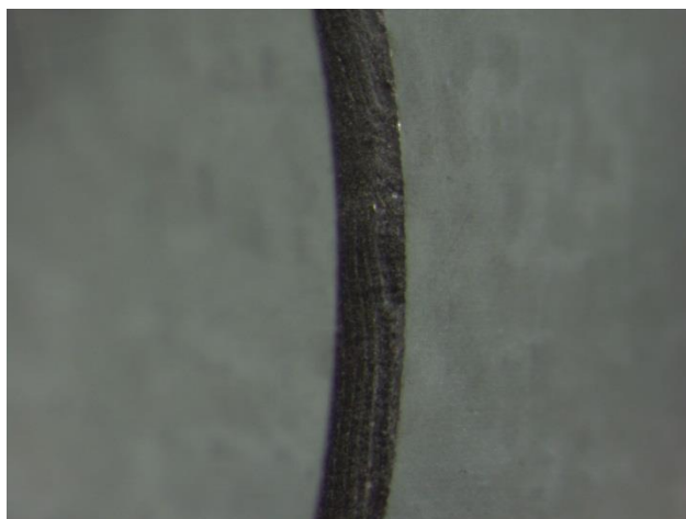
PICTURE 9: Picture of the edge of cutting for the Ref B on the 2.0mm thick SS
