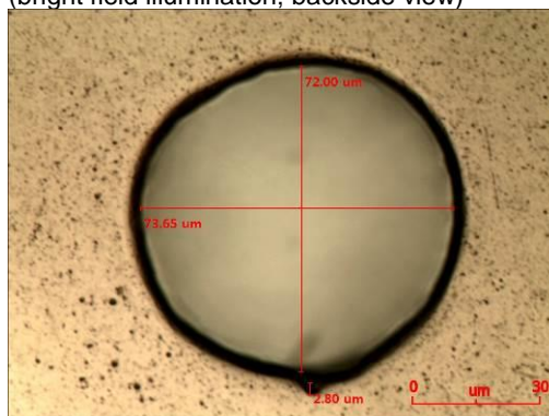
PICTURE 6: Microscope image of the drilling sample. (bright field illumination; backside view)
