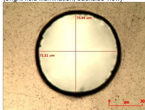
PICTURE 10: Microscope image of the drilling sample. (bright field illumination; backside view)
