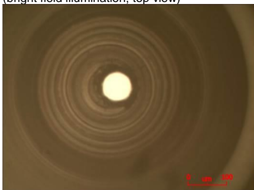
PICTURE 3: Microscope image of the drilling sample. (bright field illumination; top view)
