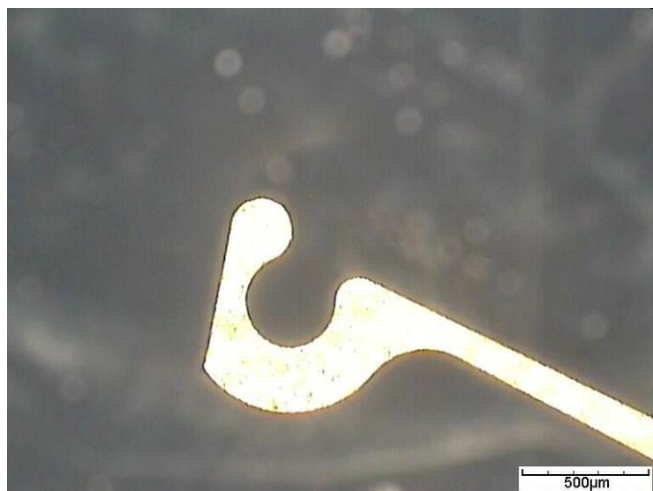
IMAGE 20: Crochet, Face avant, laiton 0.45mm
