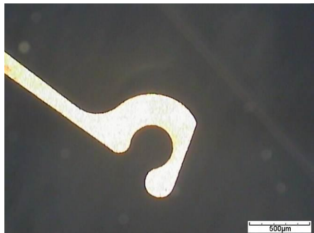
IMAGE 17: Crochet, face avant, CuBe 0.4mm
