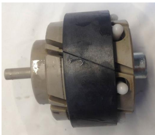
FIGURE 4: Pictures of a cut ring on (left) and out of the specific holder (right)
