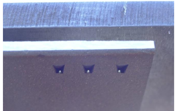
FIGURE H: Close-up on the diffusers, showing the 0.25mm holes that were drilled inside.
