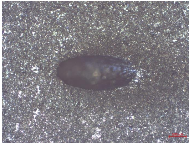
FIGURE M: Front side of a 0.35mm hole.
