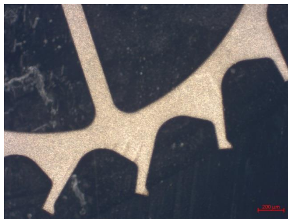
PICTURE 18 and 19: Picture of the teeth for escape wheel 6, frontside at left and backside at right
