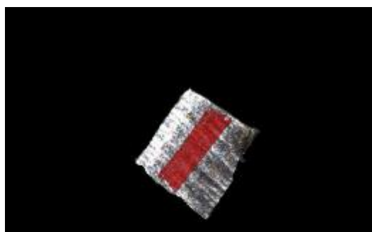
PICTURE 30: Roughness measurement for a tooth of the escape wheel
