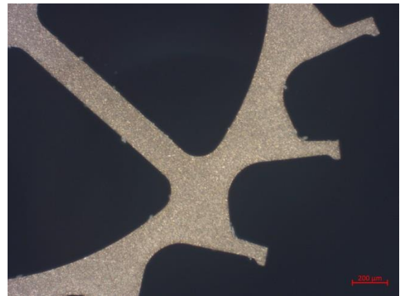
PICTURE 6 and 7: Picture of the teeth for escape wheel 2, frontside at left and backside at right
