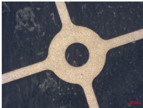
PICTURE 16 and 17: Picture of the center hole for escape wheel 6, frontside at left and backside at right
