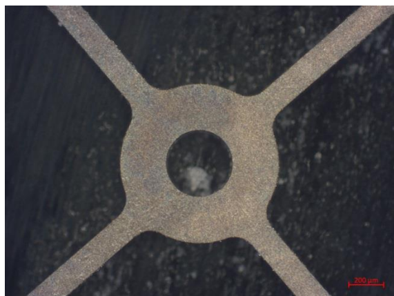
PICTURE 10 and 11: Picture of the center hole for escape wheel 4, frontside at left and backside at right
