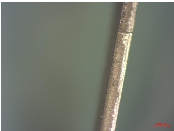
PICTURE 8 and 9: Picture of the side of escape wheel 2 at left and one of its teeth at right
