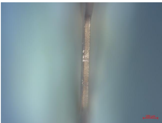
PICTURE 20 and 21: Picture of the side of escape wheel 6 at left and one of its teeth at right
