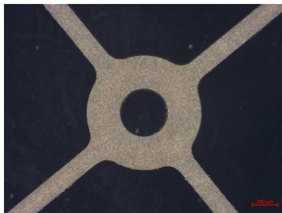
PICTURE 10 and 11: Picture of the center hole for escape wheel 4, frontside at left and backside at right
